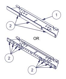
Attach the MultiFast Optim bracket (1) to the top of the profile with 12 Pisko sheet metal screws of stainless steel (3). Fasten the screws according to the pattern shown in the drawing. **Do not overtighten!**
