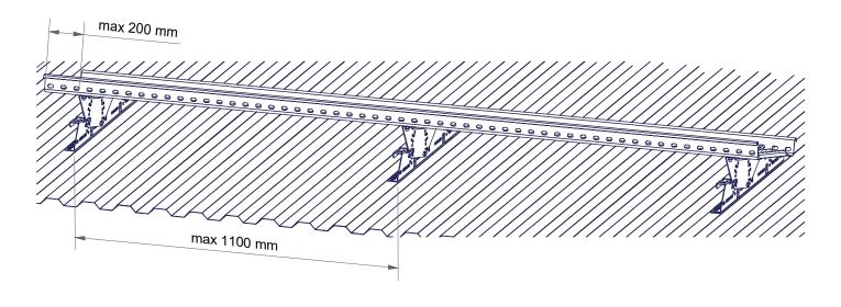
The extension of the walkway (7) shall be done by overlapping (min 2 crossbars) and securing the connection from both sides with two M8x16 flange bolts (8) and M8 flange nuts (9).
