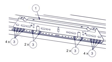
The mounting angles and corresponding mounting holes. The mounting holes are
