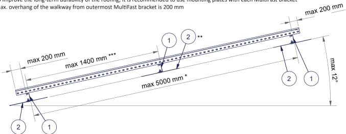
Install the mounting plates for waterproofing membrane roof (2) according to the assembly instruction of the mounting plate on waterproofing membrane roof.
