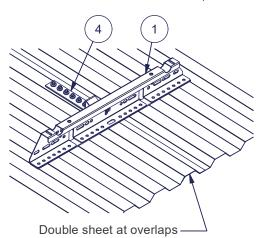
**B**: 2 Fixing rods (4) / Multifast bracket on single aluminium sheet.
