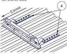
Attach the walkway (3) to MultiFast brackets (1) with flange bolts (5) (2 pcs / bracket)
