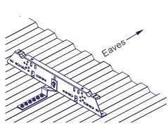
In areas of heavy snow loads it is recommended to attach roof walkway to roof with more than minimum amount of steel roof fixing rods. 2 fixing rods / MultiFast bracket can also be used.
