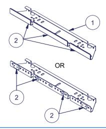
Attach the MultiFast Optim brackets (1) to the Pisko walkway (3) with flange bolts (4) (2 pcs / bracket).
