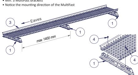
Place the walkway to roof. Roof seam is inserted into one of the two mounting holes on the MultiFast Optim bracket.
