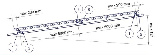
Multi-purpose standing seam brackets (5) are mounted on lock- / tinsmith-seam with SG tightening clamps (6). Attach brackets and tightening clamps to the seam. Correct tightening torque will spread out the tightening clamp a bit, in order to create a tight long-lasting connection. Tightening torque of fixing bolt (7) is 18 N/m.
