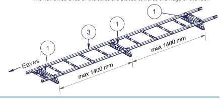
Attach MultiFast Optim (1) to the ladder (3) with 2 x MultiFast stile bracket Optim (4). Insert the hook end of the stile bracket to oval hole on top of the MultiFast bracket, turn it around the stile of the ladder and fasten it with flange bolt (5). The MultiFast bracket should be installed as close as possible to the underside of the rung, to ensure good usability of the ladder.
