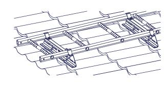
The ladder is attached to the roof with a steel roof fixing rod for MultiFast Optim (6).
