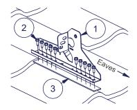
The brackets (1) are installed on top of the extension where two metal sheets overlap:
