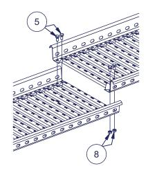
Maximum protrusion of the walkway from the outermost bracket is 200 mm.
