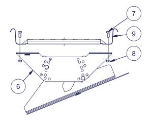
The extension of the walkway shall be done by overlapping and securing the connection from both sides with two M8x16 bolts (7) and M8 nuts (8).
