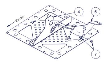
The most common roof pitches and corresponding holes.
