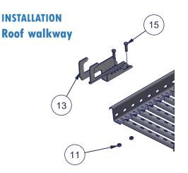
Set the slip guard to walkway side at the bottom of the groove. Put two M8x30 bolts through slip guard to walkway holes.
