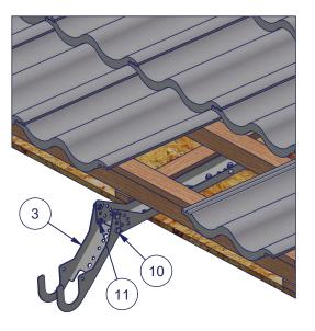
Fix the slip guard to the bracket with four M8x16 hexagon bolts and nuts.
