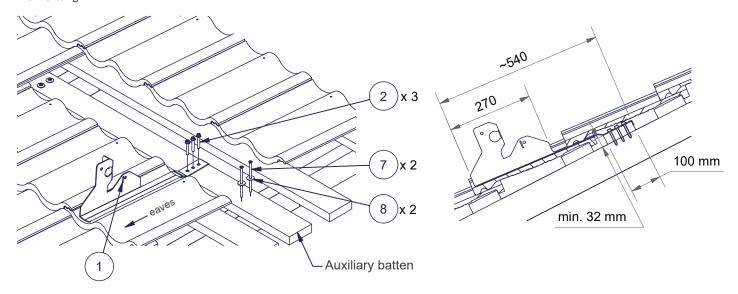
Always use at least three bracket per continuus lenght. Distance between brackets max. 1000 mm
