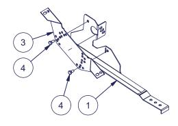
Use the slope adjustment plates to adjust the roof walkway to the horizontal level. The most common roof pitches and corresponding holes are shown in the figure.
