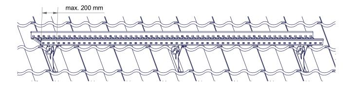
The extension of the walkway shall be done by overlapping and securing the connection from both sides with two M8x16 bolts (4) and M8 nuts (6).
