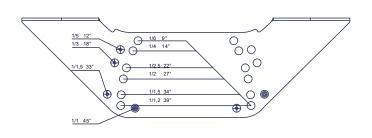
Attach walkway (5) to each adjustment plate (3) with two M8x16 bolts (4) and two M8 nuts (6).
