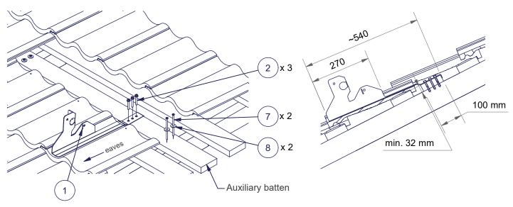
Always use at least three bracket (1) per continous lenght. Distance between brackets max. 1000 mm
