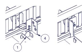
Install the Pisko SnowDefence 150 Compact snow fence (3) to the bracket (1) with the drainage holes in the fence profile facing down.
