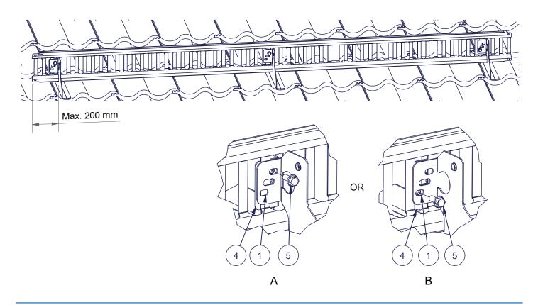
Fence extension shall be made with 2 flange bolts (5) and nuts (7).
