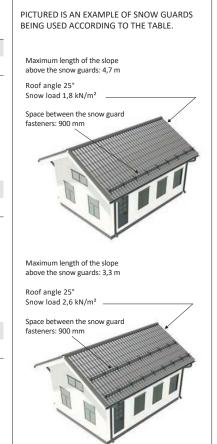
Pisko Snow Guards are capable of bearing a load of at least 5 kN/m, in the direction of the inclined roof. By following the values in the table these requirements are fulfilled.
