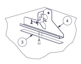
Install Bracket (4) to mounting plate bolt (2) with stainless steel M10 flange nut (5).
