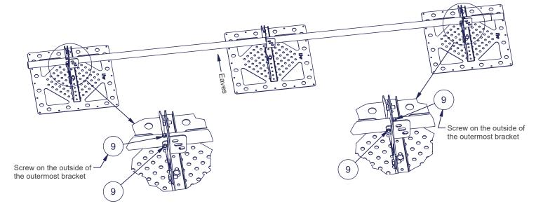
The extension of the pipes shall be done by sliding the pipe end with solid reducer inside the adjacent non-reduced pipe and fixing pipe fixing screws (9) (2 pcs/joint) through the pipe connections.
