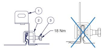
Install the Snow Rake (4) to the brackets (1) with M8x16 (5) flange bolt (can also be attached with M8x16 bolt and washer). Max. distance between the brackets is 1200 mm.
