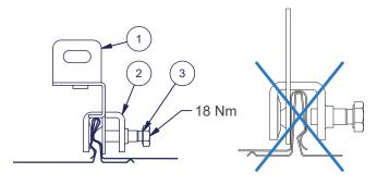
Install the Snow Rake (4) to the brackets (1) with M8x16 (5) flange bolt (can also be attached with M8x16 bolt and washer). Max. distance between the brackets is 1200 mm.
