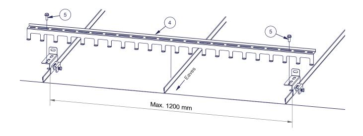
Install the Snow Rake on the roof so that the fingers do not overlap the seams. If this can't be avoided, bend the finger 90° upwards so that it doesn't touch the seam. Recommended height between the Snow rRke and roof surface is 5 - 10 mm. Max. protrusion of the Snow Rake from the outermost bracket is 200 mm.
