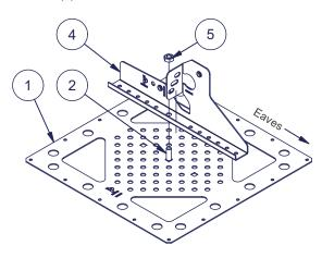
Install the snow fence (6) to the brackets (4) with the drainage holes in the fence profile facing down.
