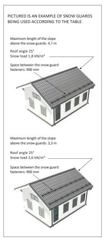
Pisko Snow Guards are capable of bearing a load of at least 5 kN/m, in the direction of the inclined roof. By following the values in the table these requirements are fulfilled.
