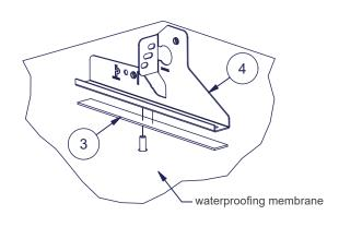
Install Bracket (4) to mounting plate bolt (2) with stainless steel M10 nut (5).
