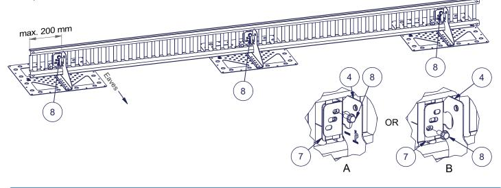
Attach the outermost fixing clamps (7) to the snow fence with fixing screws (9) in each continuous length.
