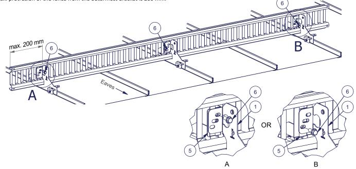
Attach the outermost fixing clamps to the snow fence with fixing screws (2) in each continuous length.
