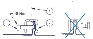
At least 3 brackets per continuous lenght. Maximum distance between the brackets is 1200 mm.
