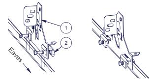
Tightening torque of the fastening bolt (3) is 18 N/m. Correct tightening torque will spread out the Tightening clamp a bit, in order to create a tight long-lasting connection. NB! The bolt of Tightening clamp must always be against the fastener, NOT against the seam.
