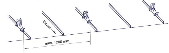
Install the snow fence (4) to the fasteners (1) with the drainage holes in the fence profile facing down..
