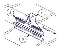
The brackets (1) are installed on top of the extension where two metal sheets overlap:
