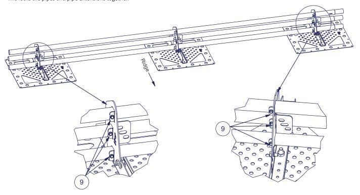
The extension of the pipes shall be done by sliding the pipe end with solid reducer inside the adjacent non-reduced pipe.
