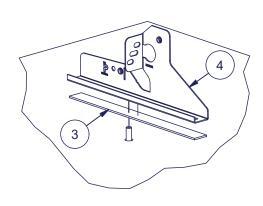
Install Bracket (4) to mounting plate bolt (2) with stainless steel M10 nut (5).
