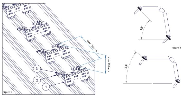
The maximum distances between steps are indicative. The positioning should be made on a case-by-case basis, taking into account the shape of the roof and usability of the access route.
