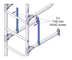
• The wall ladder legs are fastened to the eaves structure with the aid of eaves supports. Whenever possible, it is recommendable to use them. Eaves supports are to be used when the length of the wall ladder legs exceeds 400 mm. The purpose of the eaves supports is to support the ladder under vertical loading. The eaves support is fastened to the wall ladder leg with an M8x30 hexagon screw and M8 hexagon nut and to the eaves with e.g. 7x40 mm HVAC screw (2 per eaves support).
