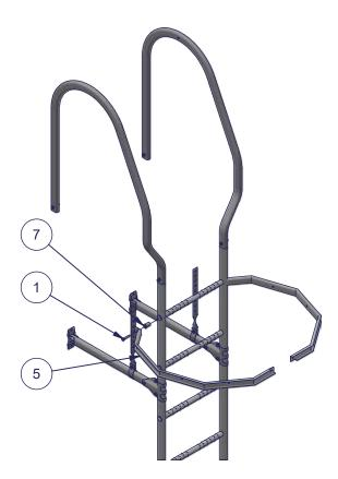
Before installing safety cage wall ladder are assembled according to wall ladder installation intruction.
