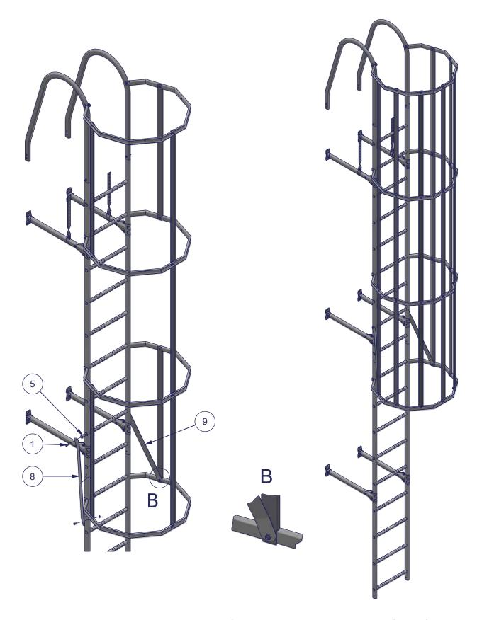
Assemble lowest rim pair vertical laths closest to the wall ladder from the lower end with M8x16 bolts and fasten left and right support lower end with the same bolts. Fasten left and right support upper end with rubber nuts and M8x40 bolts two rungs higher than lowest rim pair.
