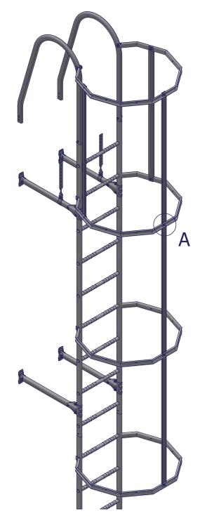
Fasten center line vertical lath pair through the rims with M8x16 bolt and nut.
