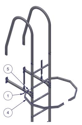
Before installing safety cage make sure that wall ladder bows are assembled as shown in the picture, in different direction compared to normal. Wall ladder is assembled otherwise like in wall ladder installation instruction.
