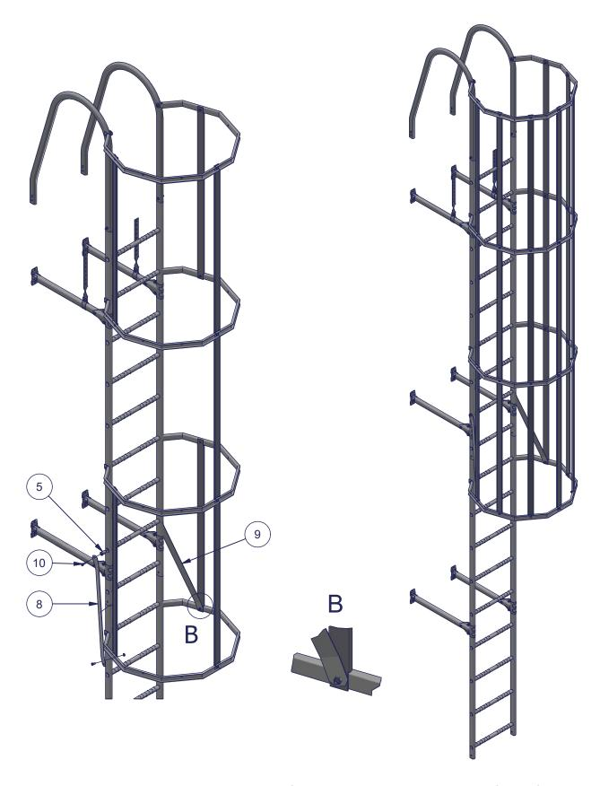
Assemble lowest rim pair vertical laths closest to the wall ladder from the lower end with M8x16 bolts and fasten left and right support lower end with the same bolts. Fasten left and right support upper end with rubber nuts and M8x60 bolts two rungs higher than lowest rim pair.
