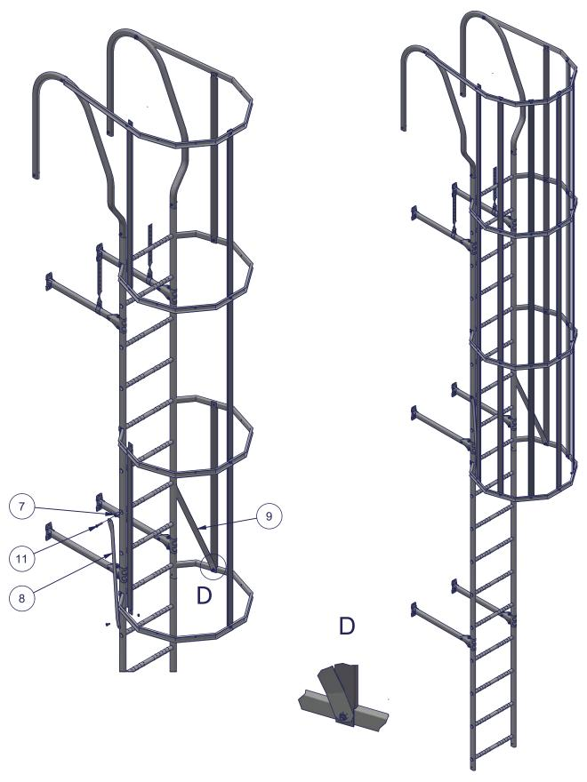
Assemble lowest rim pair vertical laths closest to the wall ladder from the lower end with M8x16 bolts and fasten left and right support lower end with the same bolts. Fasten left and right support upper end with rubber nuts and M8x60 bolts two rungs higher than lowest rim pair.
