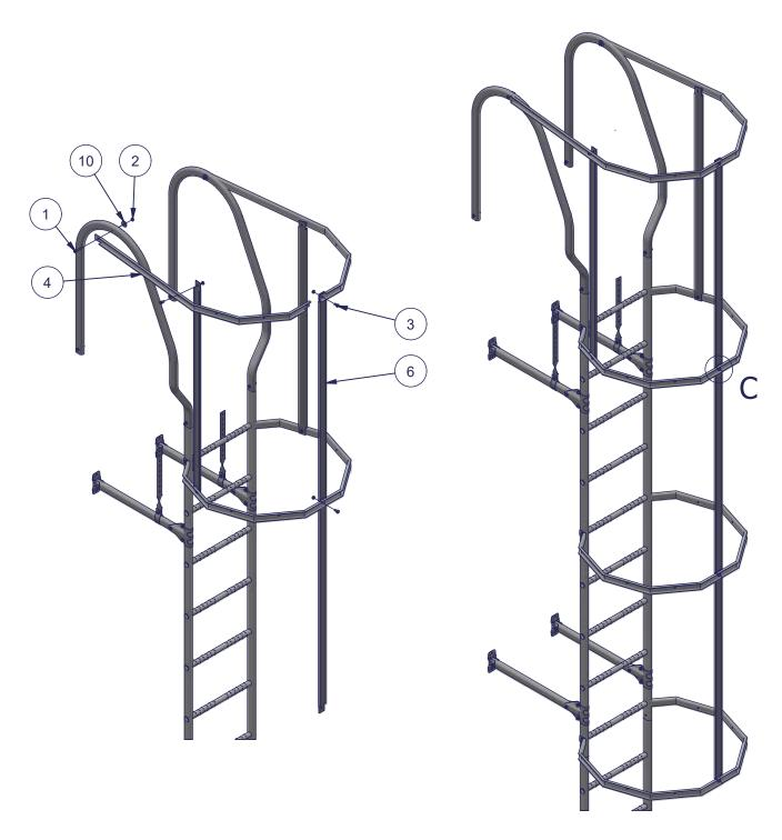
Fasten center line vertical lath pair through the rims with M8x16 bolt and nut.
