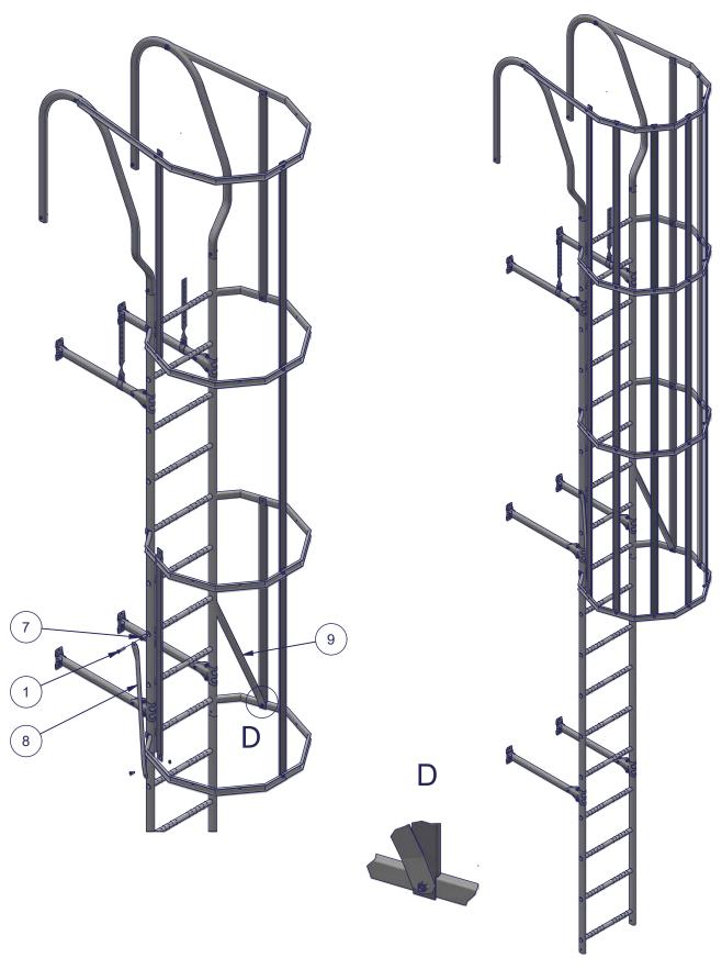
Assemble lowest rim pair vertical laths closest to the wall ladder from the lower end with M8x16 bolts and fasten left and right support lower end with the same bolts. Fasten left and right support upper end with rubber nuts and M8x40 bolts two rungs higher than lowest rim pair.
