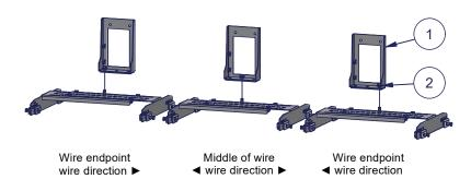
Insert SafeLine wire holder bracket (3) in the fixing support so that the holes are aligned.
