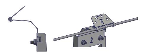
Bend the top plate of the bracket towards the lower plate. While doing this, make sure the wire stays inside the ring shaped elements of the bracket. Lock the plates together with M8 flange bolts and flange nuts. Use the mounting holes closest to the wire. The tightening torque is approx. 30 Nm, or until the surfaces are completely against each other at the point of attachment.
