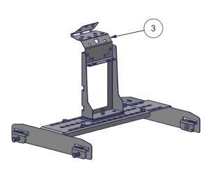
Fasten the wire holder bracket on the fixing support with M8 flange bolts (4) and nuts (5).
