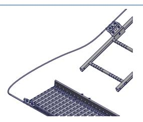
When extending the wire from a wall ladder to a roof ladder or a walkway, make sure the bend on the wire is smooth and the glider moves through the bend with ease. A bracket (1) must be installed as close as possible to the end of the wall ladder and the beginning of the roof ladder or walkway, while maintaining a smooth wire curve.
