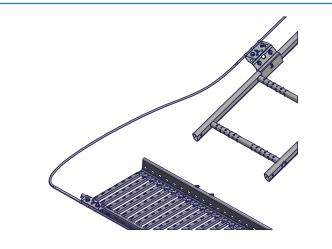
When extending the wire from the roof walkway to a roof or wall ladder, make sure the bend on the wire is smooth and the glider moves through the bend with ease. A bracket (2) must be installed as close as possible to the end of the roof walkway and the beginning of the ladder, while maintaining smooth wire curve.
