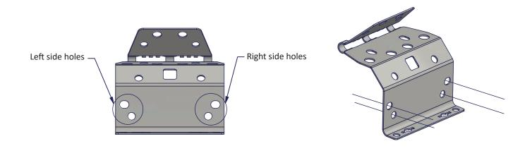
Example of using the additional attachment holes on the SafeLine wire holder bracket to install it on a walkway from other manufacturer
