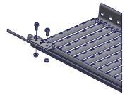
Install the remaining wire holder brackets accordingly
