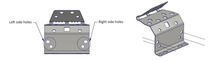
Bracket installation on a ladder which allows installation on the outside of the stile.
