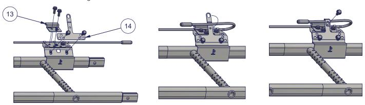
If the wire ends at the bottom of the ladder, when the ladder is in safe zone, installing the glider end stop and wire ending bracket is not mandatory. In this case, leave at least 150 mm of wire after the bottom wire holder bracket.
