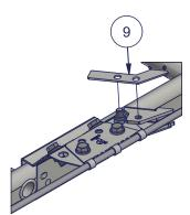
Tighten the handle (9) in it's position with M8x8 bolt on the threaded hole of the glider stopper (8).
