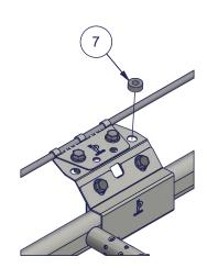
Slide the glider stopper for ladders (8) on the bracket, so that the holes in the stopper and the spacer (7) are aligned. The stopper is correctly aligned when P-mark is towards the front. The wire will run through the fork of the glider stopper.
