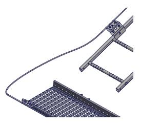
When extending the wire from a roof ladder to a wall ladder or a walkway, make sure the bend on the wire is smooth and the glider moves through the bend with ease. A bracket (1) must be installed as close as possible to the end of roof ladder and the beginning of the wall ladder or walkway, while maintaining a smooth wire curve.
