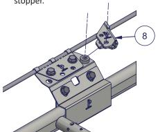
Place the handle for the glider stopper (9) on the glider stopper (8) so that the holes are aligned.
