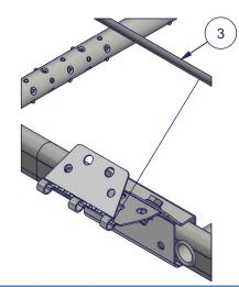
Maximum distance between two brackets on a roof ladder is 1500 mm.
