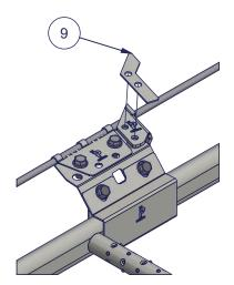
Lock the glider stopper (8) and the handle (9) in place with M8x30 flange bolt (10) from the front and an M8 nyloc nut (11) from the back.
