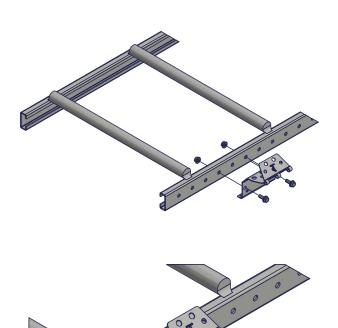
Bracket installation on a ladder which allows installation on the inside of the stile.
