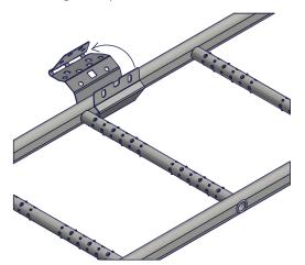
Lock the fixing piece to the wire bracket with 2 x M8 flange bolt and 2 x M8
