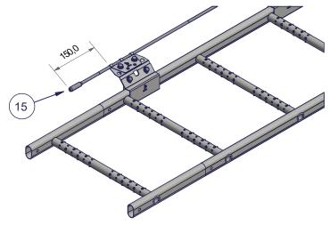
If the loose end of the wire after the last bracket has not been equipped with any factory-mounted terminal, it shall be protected with wire end protector (15) by pressing or using an alternative corresponding method.
