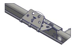
Lock the plates together with 2 x M8 flange bolts and 2 x M8 flange nuts. The tightening torque is approx. 30 Nm, or until the surfaces are completely against each other at the point of attachment.
