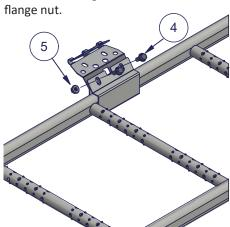
When inserting the wire inside the bracket (1) make sure the wire is completely inside the ring shaped elements of the bracket (1). Otherwise the teeth on the bracket (1) might not align correctly with the wire.
