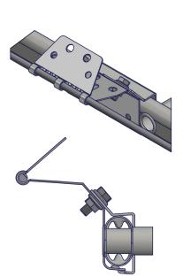
Bend open the top plate of the bracket (1) so that the wire fits inside the ring shaped elements of the bracket (1).
