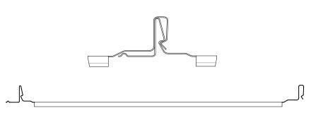
\*\*\*) Standing seam roofs according to current recommendations, using raw material of at least 0.50 mm standing seam quality (DX52D). Seam height of the standing seam roof in the controlled test around 25 mm.
