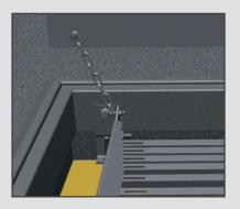
• The fire resistance class EI 60 requires placing two 30-mm layers of fire-resistant wool on top of the bottom cover.
