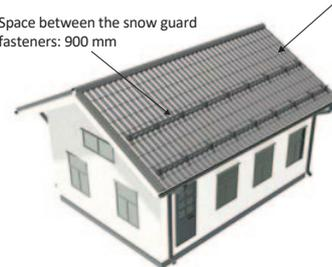
Pisko Snow Guards are capable of bearing a load of at least 5 kN/m, in the direction of the inclined roof. By following the values in the table these requirements are fulfilled.
