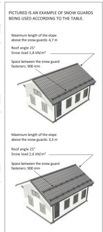
Pisko Snow Guards are capable of bearing a load of at least 5 kN/m, in the direction of the inclined roof. By following the values in the table these requirements are fulfilled.
