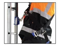
3. The carriage is designed to follow the user lightly without the user having to lean backward. When climbing, keep the fastening point of the harness as close as possible to the rail. This is emphasised when descending, and is best done by holding on to the ladder stiles (vertical posts) by hand.
