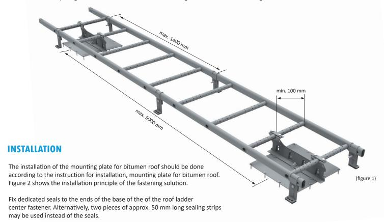
Fix the roof ladder center fastener to the mounting plate by using one hot dip galvanized M10 nut.
