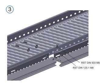
Install the subsequent horizontal rails ensuring that the neck mounting at the other end of the rail is placed in the hole at the end of the next rail. Secure the extension point with M8x8 RST screws. Also attach each horizontal rail to the roof walkway with four M8x20 screws and nuts as described in step 1.
