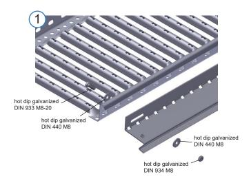
Attach the first horizontal rail to the roof walkway with four M8x20 screws and nuts through every third oval hole on the horizontal rail at approximately one meter intervals. Use a washer both between the screw head and nut. Note: If a fixed carriage stopper is used, see also section 2.
