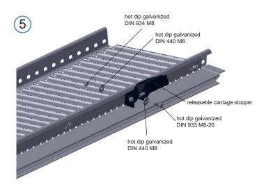
Mount releasable carriage stoppers at a minimum distance of 320 mm from the horizontal rail end.
