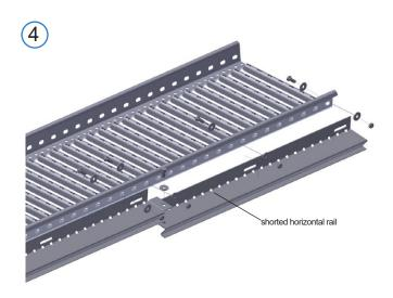
Shorten the last rail as necessary. Attach the end of the rail through the last oval hole. If the last intact oval hole of the horizontal rail is over 150 mm away from the rail end, drill the last hole at a distance of approx. 70 mm from the rail end.
