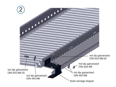
Mount fixed carriage stoppers to the horizontal rail while fastening the outermost fastening screw on the rail. Secure the attachment by placing another bolt in the tapped hole of the rail or, if necessary, by drilling an attachment hole for an M8x20 screw and nut.
