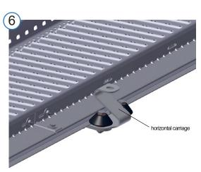
Finish by installing carriage stoppers at the end of the rail (see section 2 or 5). If mounting fixed carriage stoppers at both ends of the profile, remember to install the horizontal carriage on the rail before mounting the last stopper.
